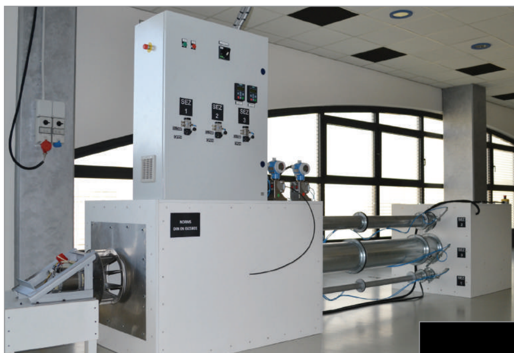
Testing Machine norms UNI EN ISO 5801
